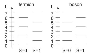
Figure 1: The allowed states for parahydrogen (S=0) and orthohydrogen (S=1) molecules for possible Fermi-Dirac or Bose-Einstein statistics for protons.
